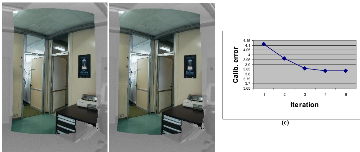
(a) (b) Laboratory 030 before (a) and after (b) calibration tuning and evolution of calibration error (c)
