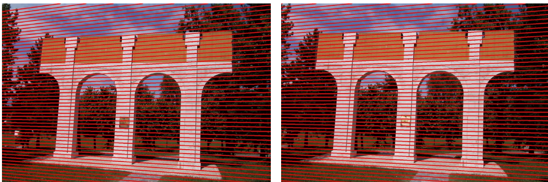
(a) (b) Figure 5-5: Epipolar lines in two intensity images of the arches
