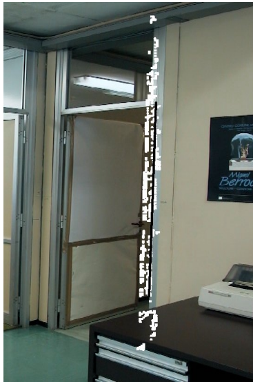
Figure 4-8: The original detected segment (black) and the re-projected 3D points in its neighbourhood (white)
