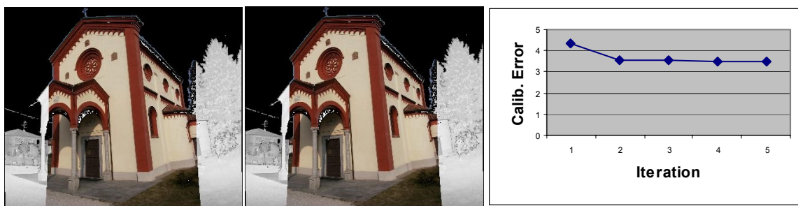
(a) (b) Church Barza before (a) and after (b) calibration tuning and evolution of calibration error (c)
