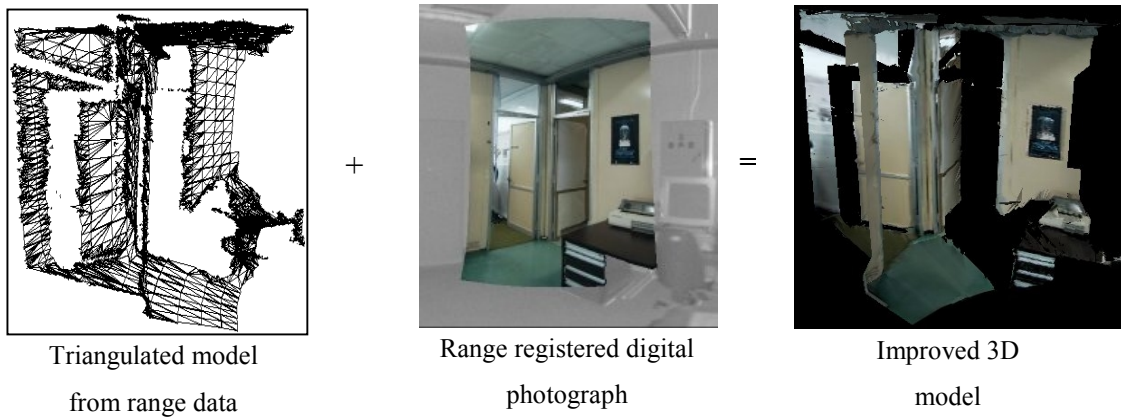
Figure 4-1: Illustration of model correction based on a single registered image
