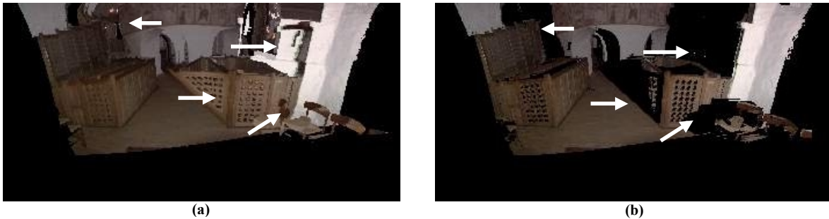
Figure 3-5: Re-projection without Z-buffering (a) and with Z-buffering (b)
