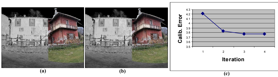
Laveno farm house before (a) and after (b) calibration tuning and evolution of calibration error (c)
