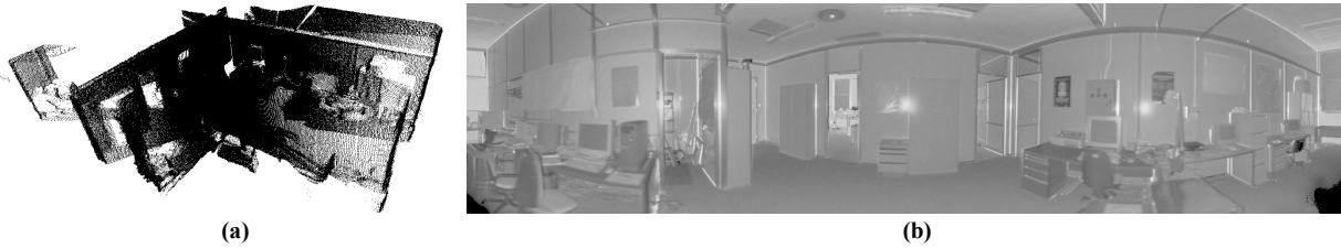
Figure 2-2: Range cloud (a) and reflectance image (b) acquired with a Riegl LMS-Z210 laser scanner (1000x240 pixels)
