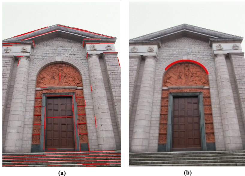
Figure 6-7: Results of line (a) and quadratic (b) detection in Laveno church image
